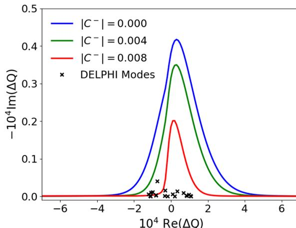
Figure 3: Reduction of stable region with increase of linear coupling. In each case the tunes are matched to  $Q_u = 0.31, Q_v = 0.32$  after coupling is introduced. If the unstable modes (as simulated in DELPHI [15]) lie outside the curve then the mode is unstable.
