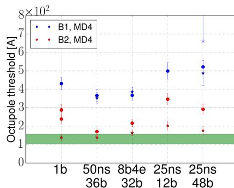
Figure 5: Octupole threshold measured for different train structures throughout 2017. The green bar indicates the predicted threshold for a single bunch with a transverse damper and considering uncertainties in the measured intensity and emittance. The cross marks the measured threshold in 2016. The dots show the measured threshold with damping time of 30 turns, while the stars represent the results obtained for a damping time of 100 turns.
