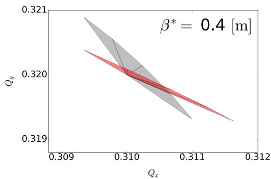
Figure 2: Tune footprint at  $\beta^* = 40\text{cm}$  for the case with octupoles only (in grey) and with octupoles and IR non-linearities (in red).
