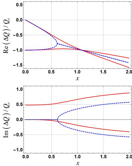
Figure 3: Solutions of the diagonalisation of the  $2 \times 2$  matrix of Eq. (7): without (blue) and with (red) the damper.
