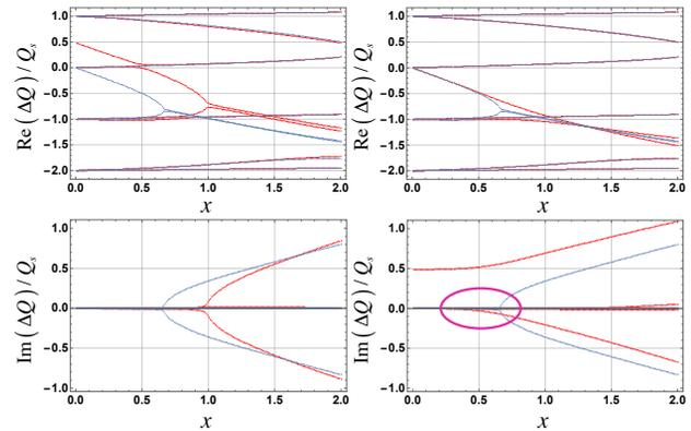
Figure 2: Usual TMCI plots (for  $f_r \tau_b = 0.8$ ) showing the real and imaginary parts of the normalised complex tune shift vs. the normalised coherent tune shift without (in blue) and with (in red) a transverse damper with  $n_d = 50$  turns: (left) reactive and (right) resistive.
