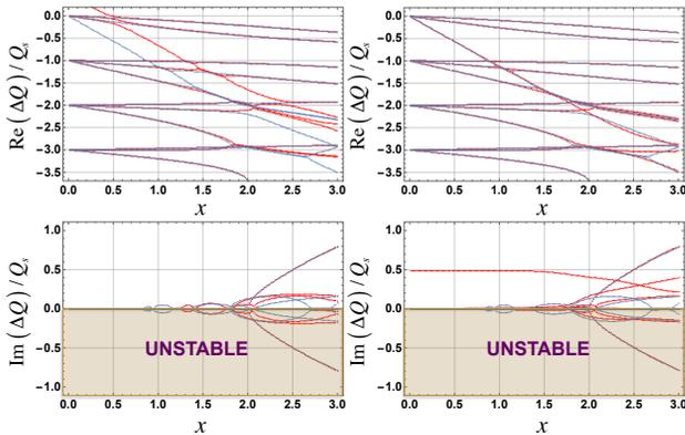
Figure 1: Usual TMCI plots (for  $f_r \tau_b = 2.8$ ) showing the real and imaginary parts of the normalised complex tune shift vs. the normalised coherent tune shift without (in blue) and with (in red) a transverse damper with  $n_d = 50$  turns: (left) reactive and (right) resistive.
