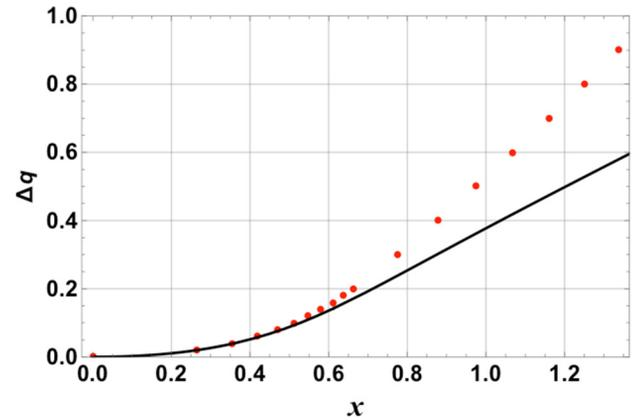
Figure 4: Required normalised tune spread to reach bunch stability vs. the normalised coherent tune shift: using the one-mode approach, leading to the usual stability diagram (black full line) and the two-mode approach from Eq. (8) (red dots) assuming an elliptical tune spread.
