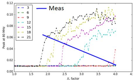
Figure 6: Simulated peak amplitude at 80 MHz, obtained from scanning the impedance factor of the 80 MHz cavities to find the value matching measurements (in blue) for different number of bunches (dotted lines).
