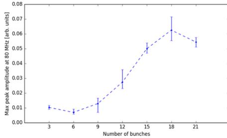
Figure 5: Maximum peak amplitude at 80 MHz in measurements of the projected beam spectrum with rf off. Values below 0.02 are below noise level.
