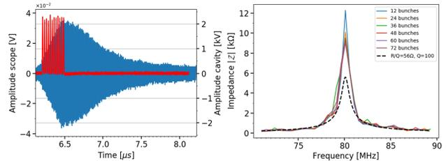
Figure 7: The left plot is an example of measured induced voltage in the 80 MHz cavity (blue) together with the measured longitudinal beam profile (red). The induced voltage is deconvolved with the beam spectrum to get the cavity impedance in the right plot (for one cavity).
