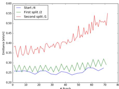
Figure 2: Measured longitudinal emittance blow-up along the batch during double splittings with the three 80 MHz cavity gaps open.
