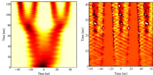
Figure 1: Double splittings at PS flat-top from  $h = 21$  to  $h = 84$ . During this manipulation the beam is split from 18 bunches to 72 bunches with 25 ns bunch spacing (left). Bunches present a 80 MHz structure during the second splitting with three 80 MHz cavity gaps opened (right).
