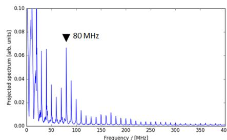
Figure 4: Measured beam profile modulation with rf off in frequency domain. The projected spectrum corresponds to the maximum amplitude of the spectrum modulation.
