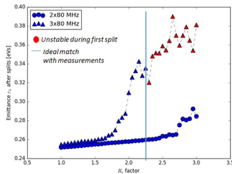
Figure 3: Maximum emittance along the batch in particle simulations, scanning the 80 MHz cavity impedance factor with two or three gaps open. The match with measurements is the vertical blue line.
