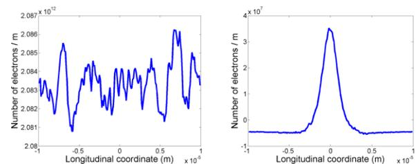
Figure 2: Comparison of magnitudes between shot noise (left) and modulation signal (right) in density distribution of electrons.
