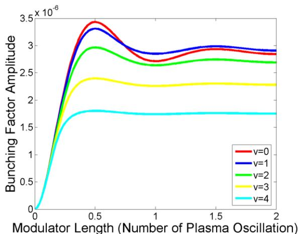
Figure 6: Amplitude of bunching factor for various longitudinal velocities of ion as a function of modulator length. The ion velocity is in unit of electron longitudinal velocity spread [9].
