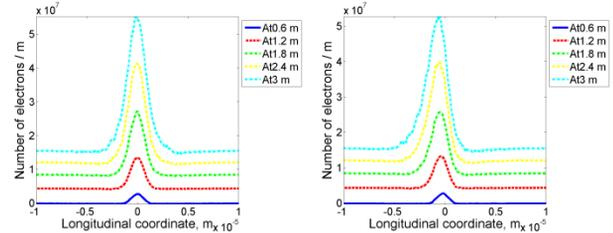
Figure 5: Longitudinal density modulation by stationary (left) and moving (right) ion at the center of the Gaussian electron beam in quadrupole beam-line.
