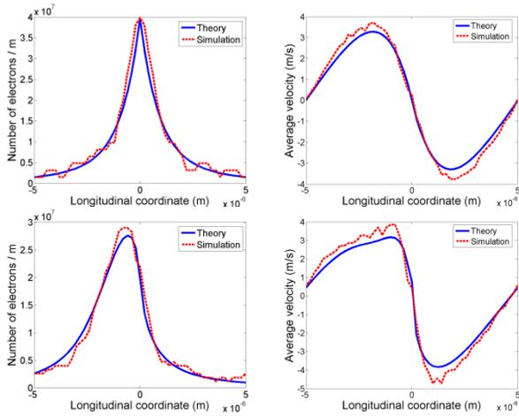
Figure 3: Comparison of theory and numerical simulations of density (left) and velocity (right) modulation by stationary (top) and moving (bottom) ion with respect to uniform electron cloud.
