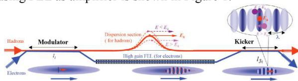
Figure 1: Schematic of coherent electron cooling concept.
