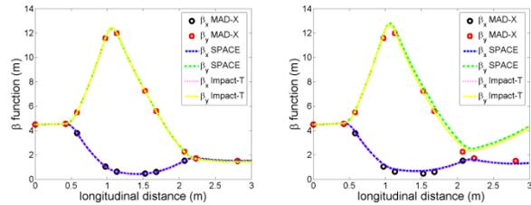
Figure 4: Comparison of transverse  $\beta$  function evolution in quadrupole beam-line using MAD-X, SPACE and Impact-T, with space charge turned off (left) and on (right).
