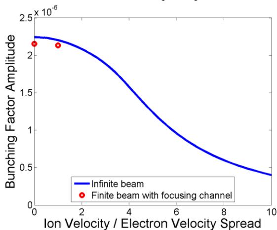
Figure 7: Comparison of amplitude of bunching factor between theory and simulation for various longitudinal velocities of ion at the exit of modulator section (a quarter plasma oscillation). The ion velocity is in unit of electron longitudinal velocity spread [9].
