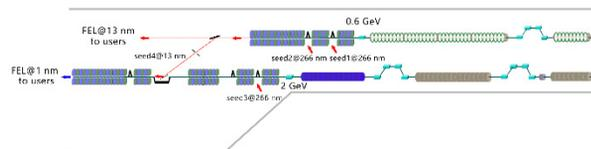
Figure 4: Proposal for testing the two-linac based two-stage EEHG at SXFEL.
