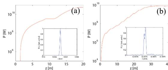
Figure 3: FEL gain curves in the radiator of the first stage (a) and the radiator of the second stage (b).
