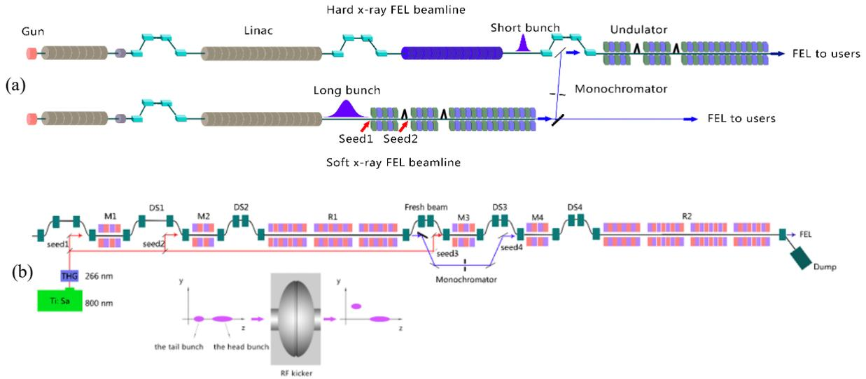
Figure 1: Layouts of two scenarios for the two-stage EEHG: (a) two-linac based two-stage EEHG, (b) double-bunch based two-stage EEHG.
