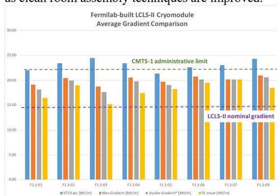
Figure 2: Cavity average gradient in the CM.
