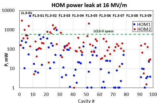
Figure 7: HOM power leak at 16MV/m.
