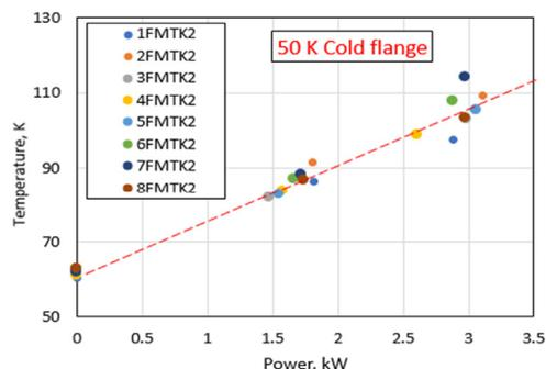
Figure 6: Temperature of the  $50\text{K}$  flange vs. RF power, measured at F1.3-09 cryomodule test.
