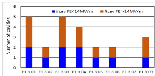
Figure 5: Number of cavities with detectable Field Emission per cryomodule tested.
