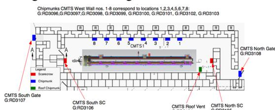
Figure 4: Layout of radiation and dark current diagnostics in the cave.
