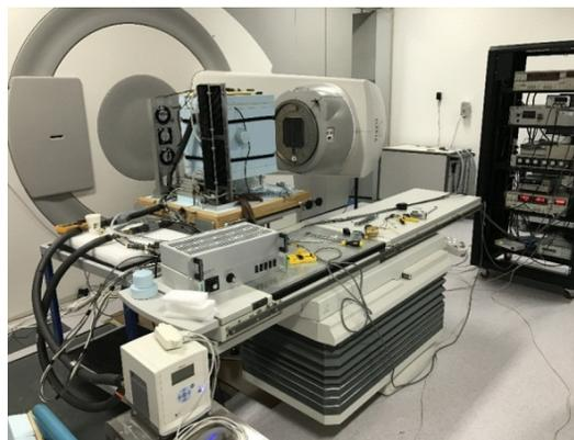
Figure 1: NIM water calorimeter for the primary standard study of absorbed dose to water of the photon beams.
