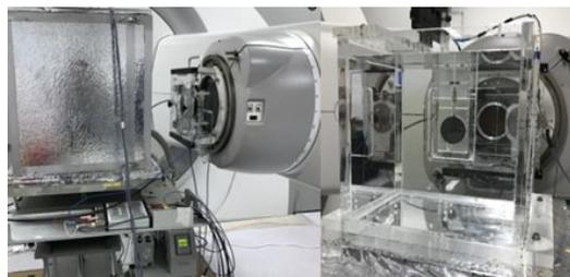
Figure 2: BIPM graphite calorimeter and the pancake chamber in the water phantom for NIM-BIPM comparison.
