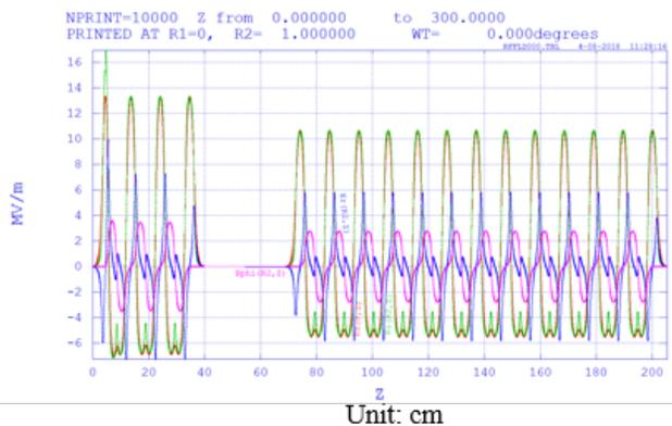
Figure 7: The longitudinal electric field distribution with beam loading.
