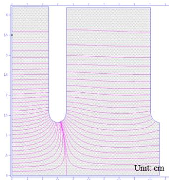
Figure 4: The longitudinal electric field distribution along the beam direction.
