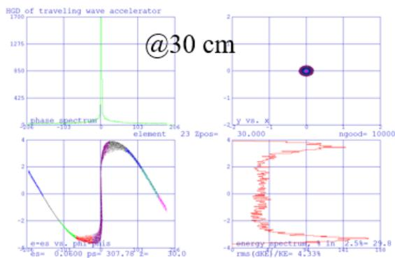
Figure 8: The velocity modulation of the particles after prebuncher.
