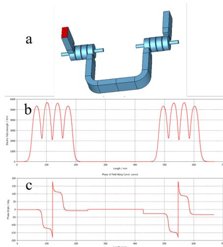
Figure 5: a: Layout of the linac; b: The longitudinal electric field distribution along the beam direction; c: The phase change between two linacs.
