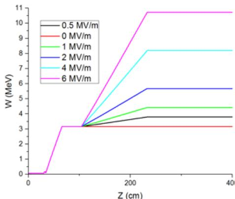
Figure 10: The energy vary with the RF power.
