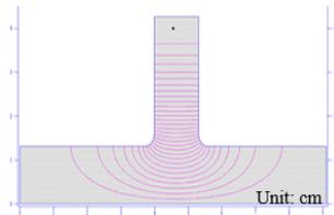
Figure 3: The electric field configuration of  $\pi$  mode of pre-buncher.
