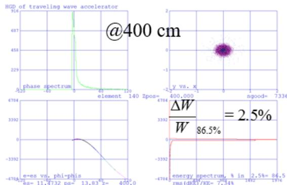
Figure 9: The energy spread of the particles, phase width and beam spot.
