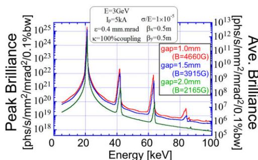
Figure 2: Example of the X-ray spectrum from very-short-period undulator ( $\lambda_u=4\text{mm}$ ,  $L=1\text{m}$ ) at ILC.
