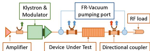
Figure 1: Schematic layout of the test setup.
