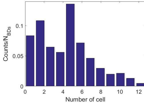
Figure 5: BD location in the RF structure.
