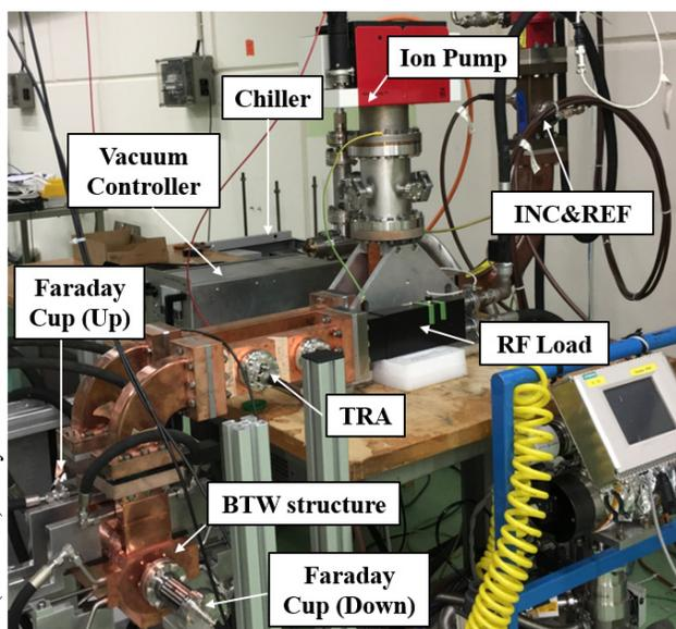
Figure 2: Picture of the test bench at S-box. Structure, diagnostics, vacuum and cooling system are labelled.
