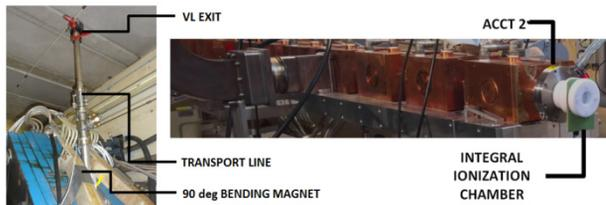
Figure 2: The vertical extraction line of the low energy proton beam (left) and the medium energy extraction point with the second ACCT device and the integral ionization chamber (right).
