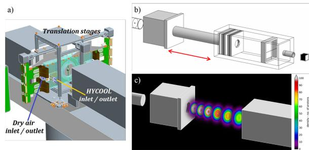
Figure 5: a) Integration area of VELO b) GEANT4 simulation of passive delivery system [10] c) Beam density profiles
