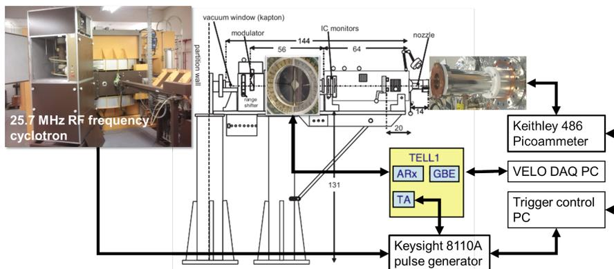
Figure 2: Synchronization of the readout of the VELO detector and the Faraday Cup optimized for the integration at the CCC proton beam line. A master trigger regulates the output of the pulse generator synchronized to the RF frequency of the cyclotron for generating VELO readout triggers and controls the picoammeter measuring the beam current by the FC.
