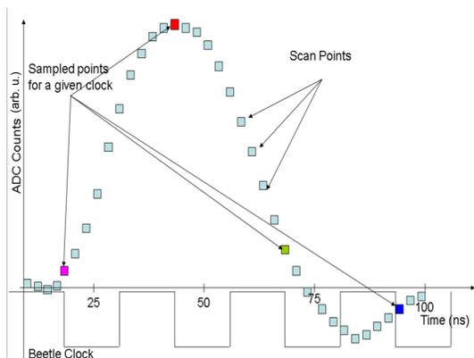
Figure 3: Sampling of the 40 MHz clock of the output pulse in the Beetle chip at different times. In the optimal case one samples at the pulse peak. [5]
