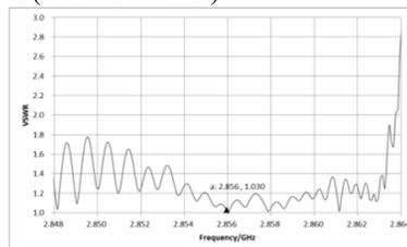
Figure 6: The measurement result of VSWR vs. frequency.
