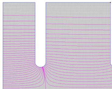
Figure 1:  $2\pi/3$  mode electromagnetic pattern with SUPERFISH.
