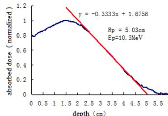
Figure 7: Result of energy test.
