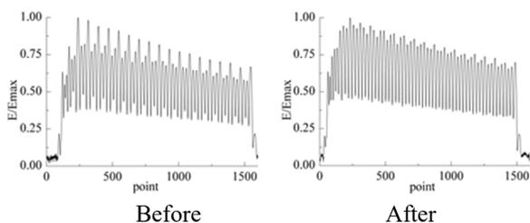
Figure 5: Travelling waves field distribution before&after tuning
