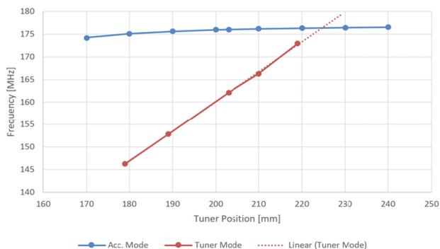
Figure 3: Measured tuner sweep of CH cavity 1 with expected tuner mode in tuning range. The Tuner position is measured from the DN100 CF flange.
