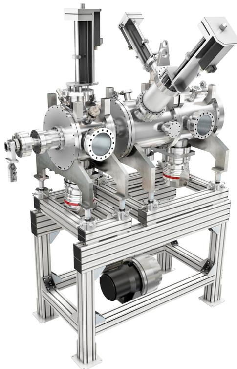
Figure 5: Setup of the Diagnostic Bench. Components on beam axis from left to right: Gate valve, ACCT, BPM, SEM, Emittance meter, BPM (hidden).
