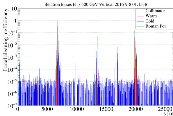
Figure 3: Measured vertical loss maps for B1 during test 2 with the collimator settings shown in Table 1.
