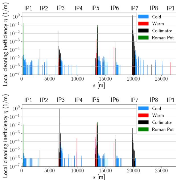
Figure 2: Simulated betatron loss maps for vertical halo configuration 1 (top) and configuration 2 (bottom) settings in Table 1 for the full ring.
