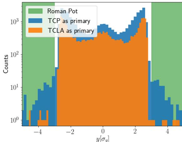
Figure 1: Comparison of the simulated beam distribution at the ATLAS-ALFA detector (A7R1) location using TCP or TCLAs as primary collimator.
