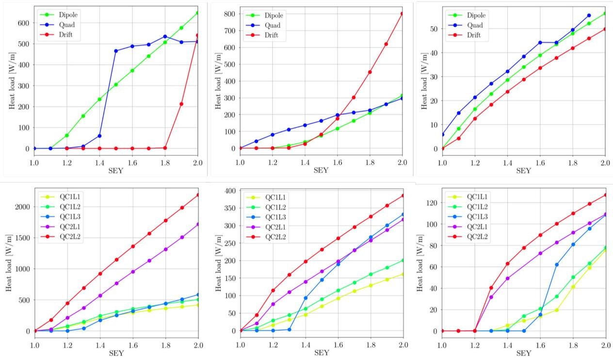
Figure 1: Heat load as a function of the SEY for the arc components (top) and IR magnets (bottom) and in the case of 2.5 ns (left), 5 ns (center) and 15 ns (right) bunch spacings.
