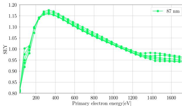
Figure 3: SEY as a function of the photoelectrons energy for the 100nm coating after the fourth activation cycle of 24 hours up to a temperature of  $250^\circ\text{C}$ .
