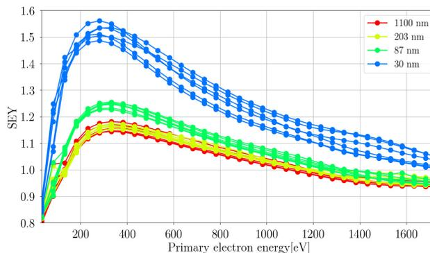
Figure 2: SEY as a function of the photoelectrons energy for all the thicknesses under study after the fourth activation cycle of 4 hours up to a temperature of  $250^\circ\text{C}$ .
