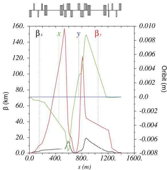
Figure 5:  $\beta$  functions and orbit for  $1.2 \times 0.15\text{m}$  flat collision optics with alternative triplet and  $40\text{ m } L^*$ .
