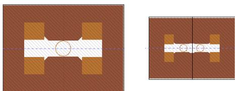
Figure 6: Transverse cross section of the FLUKA model for the dipole separator magnets: D1 (left) and D2 (right).
