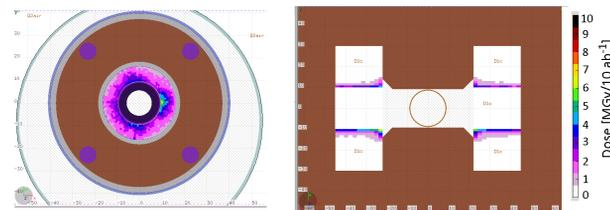
Figure 8: Transverse cross section of the magnets Q2 (left) and D1 (right), including the dose (in  $\text{MGy}/10 \text{ ab}^{-1}$ ) on the magnet coils.
