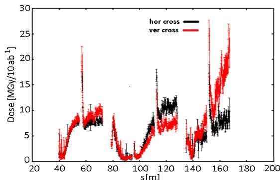
Figure 4: Peak dose profile for the flat optics ( $\theta = 114$  mrad).
