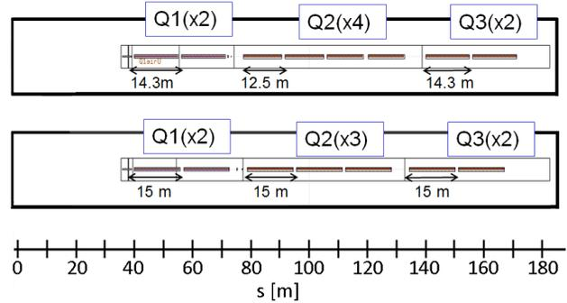
Figure 1: Comparison between the nominal (top) and the alternative triplet (bottom).
