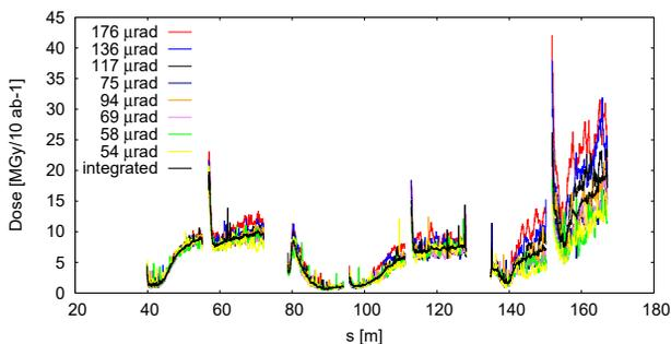
Figure 5: Peak dose profile for different crossing angles, and the total dose for varying angle runs.
