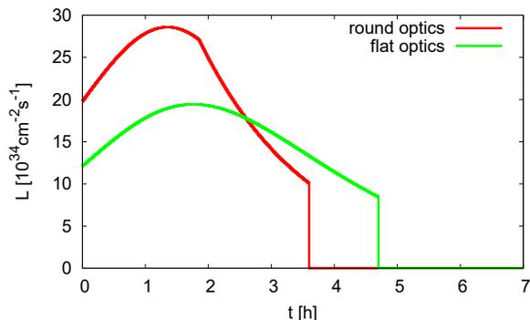
Figure 2: Luminosity evolution for round and flat beams, indicating the optimum run time for  $t_p = 4$  h.
