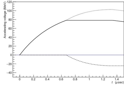
Figure 3: Voltage evolution with a constant beam loading. The solid line shows the acceleration voltage, the dashed line shows the beam loading voltage, and the dotted line shows the accelerating voltage without beam loading.
