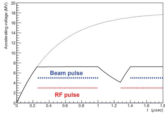
Figure 2: Voltage evolution with 2.0 A beam loading giving 7.3 MV acceleration.
