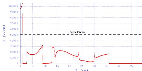
Figure 5: High Voltage Feedthrough Field Intensity Plot for  $z=0-50\text{cm}$ ,  $r=2.6\text{cm}$  and 100kV Cathode.
