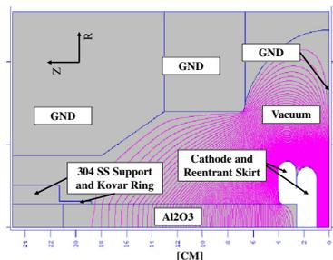
Figure 6: Cathode Standoff Electric Field Simulation.
