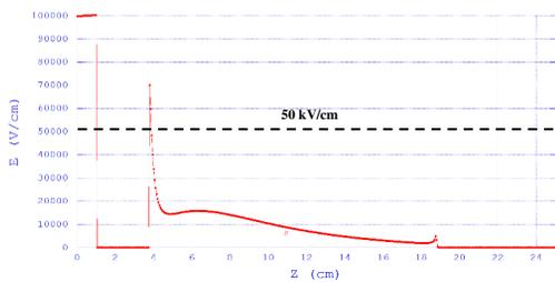
Figure 7: Cathode Standoff Field Intensity Plot  $z=0-25\text{cm}, r=1.46\text{cm}$  and 100kV Cathode.
