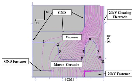
Figure 8: Clearing Electrode Ceramic Standoff Electric Field Simulation (20kV).
