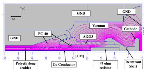
Figure 4: High Voltage Feedthrough Electric Field Simulation.
