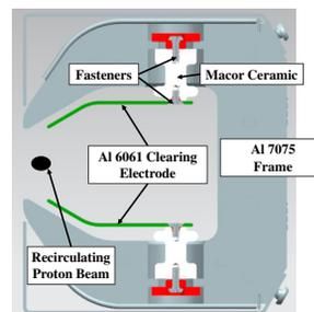
Figure 3: Clearing Electrode Mechanical Details.
