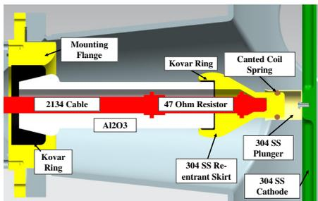
Figure 1: High Voltage Feedthrough Mechanical Details.
