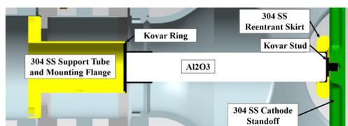
Figure 2: Cathode Standoff Mechanical Details.
