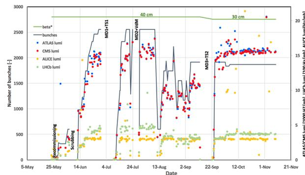
Figure 1: Different operation periods in 2017, with number of bunches and luminosities reached.
