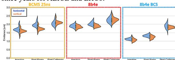
Figure 3: Emittance for the three beam types in different cycle phases: injection, ramp start and collision start.
