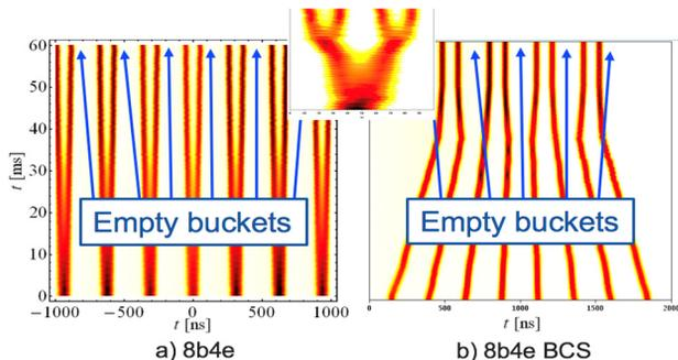
Figure 2: Beam production in the injectors: PS filled buckets alternated by empty ones, are split in 8 for the normal 8b4e; 4 double bunches separated by empty buckets are compressed before splitting in 4 for the BCS.
