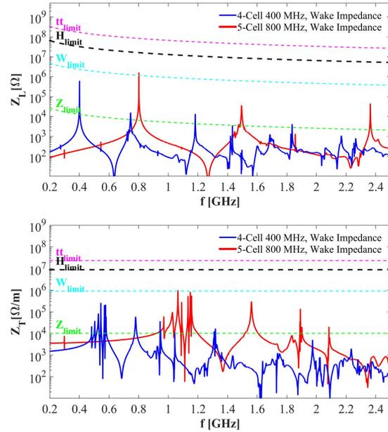
Figure 3: Comparison between the longitudinal and transversal impedance spectrum of a 4-cell cavity at 400 MHz and a 5-cell cavity at 800 MHz. A similar coaxial HOM coupler is used in both cases. The impedance thresholds set by synchrotron radiation for different energy options is plotted and normalized to the number of cavities for each case.
