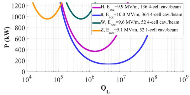
Figure 2: Forward power as a function of  $Q_L$  with optimal detuning for each energy option.
