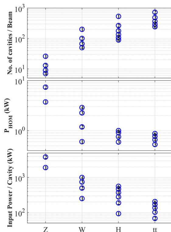
Figure 1: Dependency of number of cavities, HOM power and input power on the number of cells per cavity at 400 MHz (number of cells are shown in the circle markers). The number of cavities are calculated for  $E_{acc}=10$  MV/m. The HOM power is calculated for the BS bunch lengths of Table 1.
