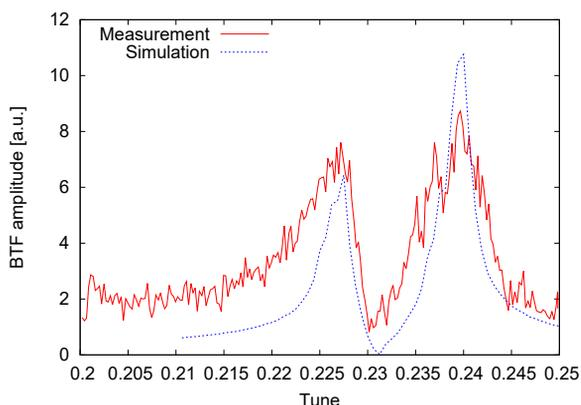
Figure 5: Comparison of horizontal BTFs between measurement and simulation.
