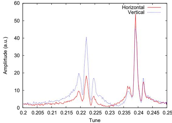
Figure 1: Measured BTF with a rebucketed beam.
