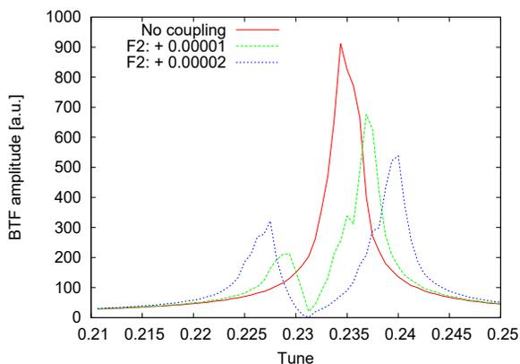
Figure 4: Simulated horizontal coupling BTFs with different skew quadrupole family settings.
