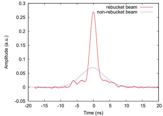
Figure 3: Measured bunch profiles w/o rebucketing.
