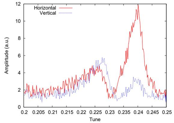
Figure 2: Measured BTF with a non-rebucketed beam.
