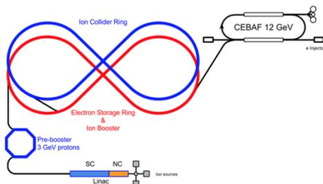
Figure 1: Layout of the alternative JLEIC design.
