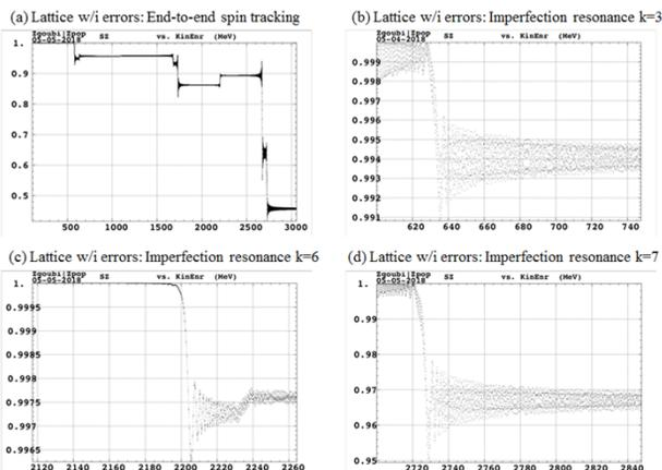
Figure 4:  $S_y$  vs KE (MeV) for the pre-booster with errors showing the energy location of imperfection resonances in addition to the intrinsic ones (a). Plots (b-d) show the strength of isolated imperfection resonances  $k=3, 6$  and  $7$ .
