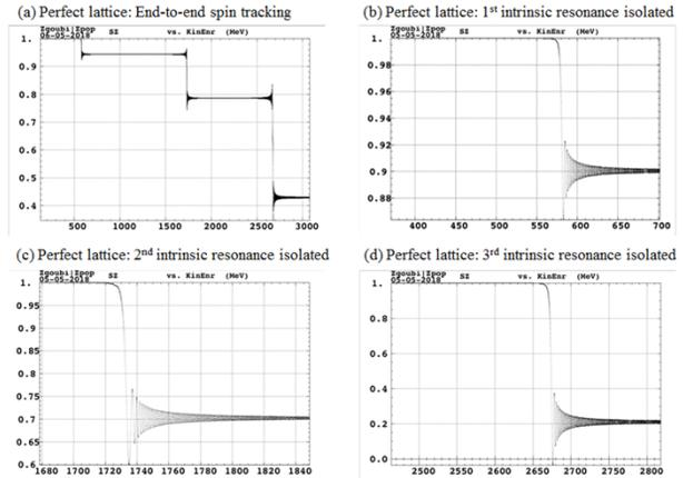
Figure 3: Vertical spin component  $S_y$  vs. proton kinetic energy KE (MeV) for a perfect pre-booster lattice showing the energy location (a) and the strengths of three intrinsic resonances (b-d). Results obtained with Zgoubi code for  $\epsilon_{y,rms} = 6\pi$  mm.mrad.
