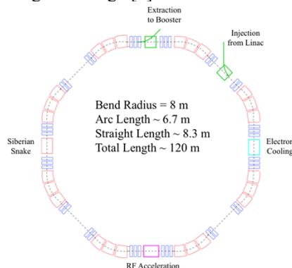
Figure 2: Layout of the octagonal pre-booster design.
