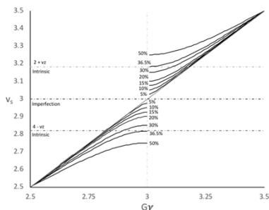
Figure 5: Spin tune vs Gy showing the spin tune gap/jump required to avoid the resonances.
