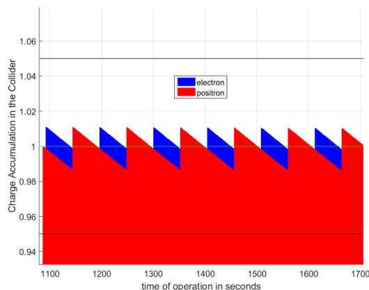
Figure 5: Top-up injection can be arranged to keep the charge imbalance to less than  $\pm 5\%$  (shown as horizontal black line). Also, the time average of both charges is kept around the full charge (shown as 1 in vertical axis).
