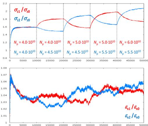
Figure 3: An illustration of bootstrapping, showing the relative bunch length and emittance fluctuations, respectively, while additional bunches are injected, where blue and red colors refer to  $e^-$  and  $e^+$  respectively.
