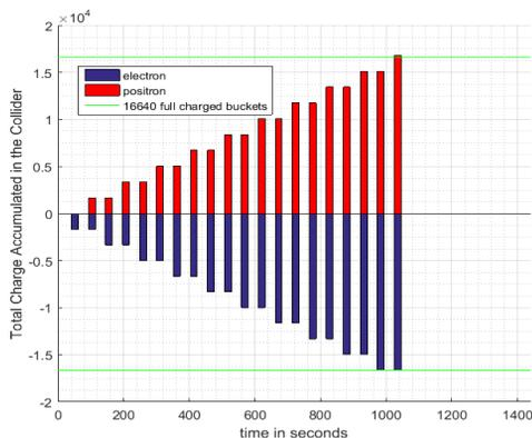
Figure 4: The first fill of the collider is complete after 1035 seconds. The vertical axis shows the total charge accumulated in the 16640 buckets where the full charge is taken as 1.
