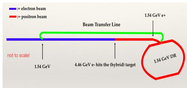
Figure 2: Positron flow scheme using the same linac as for the electrons. Notice that the positrons will be transferred back to the linac, drawn green.
