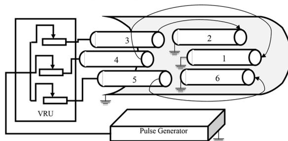
Figure 2: The kicker commutation diagram with Variable Resistance Unit (VRU).
