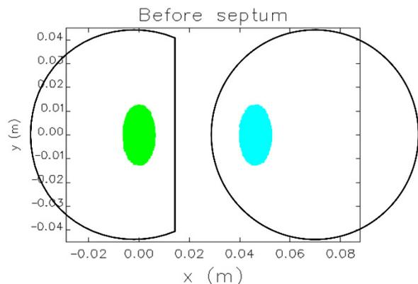
Figure 5: Beam before septum magnet. Direct channel – right.
