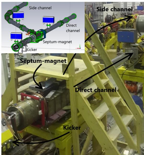
Figure 7: Experimental facility in BINP. April 2018.
