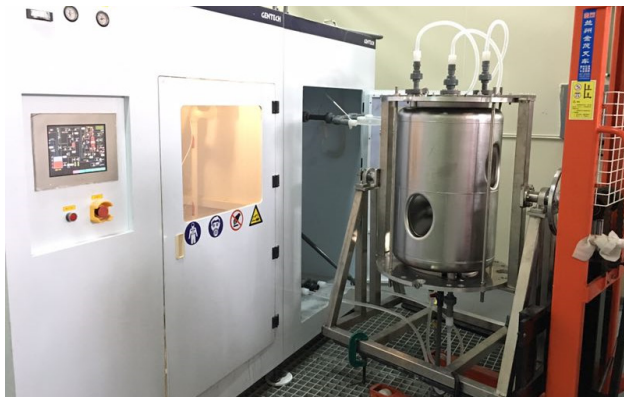
Figure 5: The BCP set-up of the double-spoke cavity.
