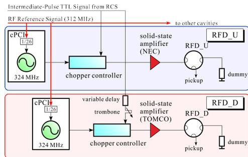
Figure 3: Schematic view of the chopper RF control system. There are two RF cavities and the parameters can be independently tuned.
