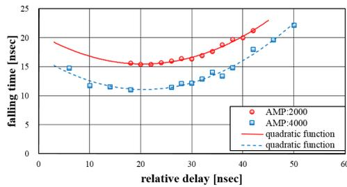
Figure 7: Results of the relative timing tune. The beam study using BPM05Y signals was performed on the two conditions with different RF amplitudes.
