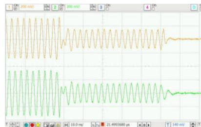
Figure 2: Oscilloscope's capture screen of the falling signal of the chopper controller. After the RF pulse falls, the short pulses with anti-phase are appeared.
