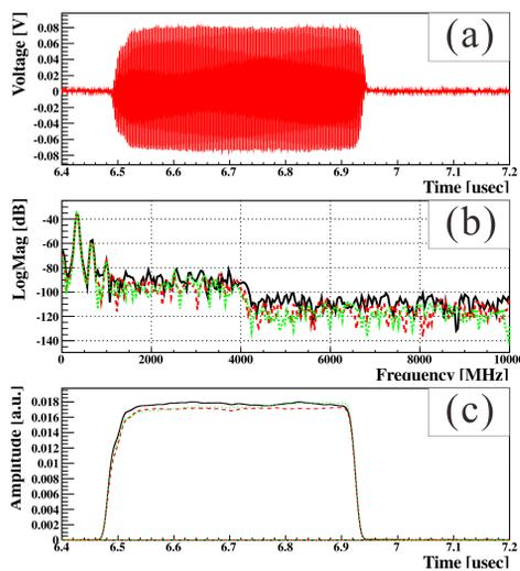
Figure 5: (a) raw signal of BPM05Y, (b) FFT analysis results and (c) intensity of the component of 324MHz, respectively.
