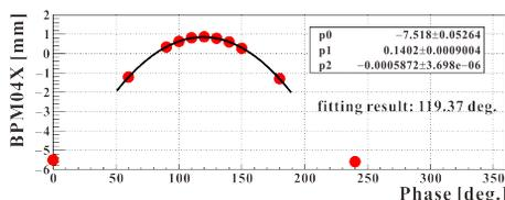
Figure 4: Results of the tune of the RF phase (RFD\_U). The optimized phase can be obtained by the largest kick-put angle.
