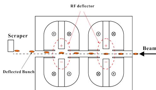
Figure 1: Schematic view of RFD. The wasted beam is kicked and led to a scraper.
