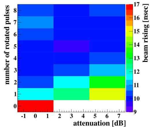
Figure 9: Results of the anti-phase function tune. When the function of anti-phase function was not used, the rising time became about 17 nsec. It was improved to about 10 nsec by optimizing the parameters of the anti-phase function.
