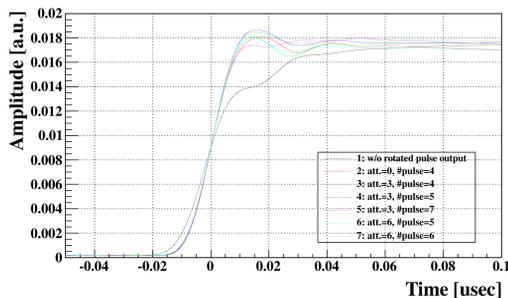
Figure 8: BPM05Y rising waveform of the intermediate-pulse beam depending on the parameters of the anti-phase function, when the only RFD\_U was driven. The time of the abscissa axis was shifted to be zero in the amplitude of 0.01. To avoid the use of the anti-phase function, the waveform of the rising shown in the black solid line has the bump on the rising. It is adversely affected by the ringing on the falling of the RF field.
