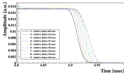
Figure 6: BPM05Y falling shape of the intermediate-pulse beam depending on the relative timing. It can be seen by the faster falling time with the relative delay of 22 nsec of the blue dash-dot line than one of 6 nsec of the black solid line and of 48 nsec the cyan long-dash line.
