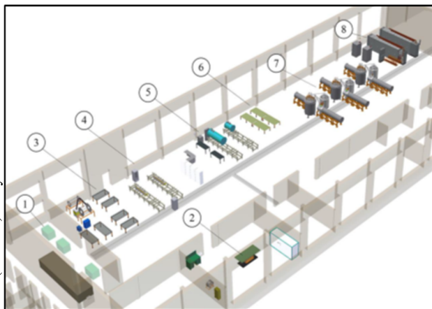
Figure 3: Schematic 3D-view of the facility halls and main equipment placement: 1 – superconducting cable; production hall; 2 – coil production hall; 3 – magnet assembling area; 4 – warm magnetic measurements; 5 – vacuum tightness check 6 – magnets assembly in cryostats; 7 – cryogenic tests at 6 benches; 8 – power converters area.
