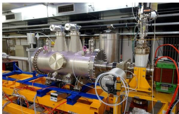
Figure 10: Installed chamber for stochastic cooling at COSY.
