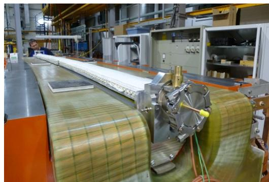
Figure 5: Installed dipole chamber with heating jackets.
