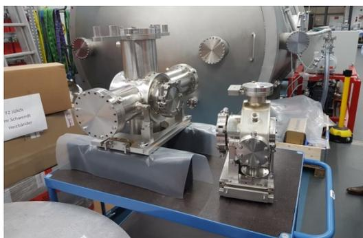
Figure 6: Manufacturing of two types of pumping bodies (DN63, DN150).
