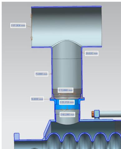
Figure 5: Cross-section through the chimney on the helium vessel.
