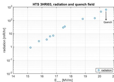
Figure 3: Radiation and quench field of 3HRI03 in HTS.
