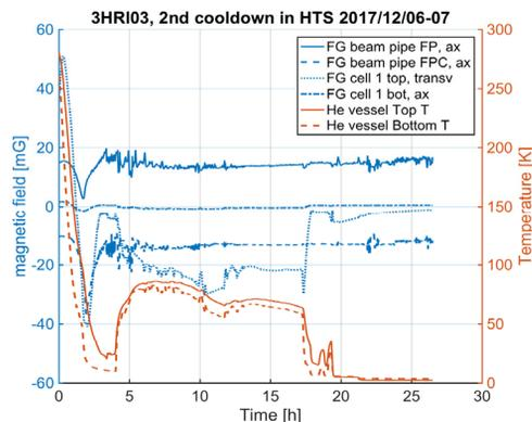
Figure 4: Magnetic fields measured by fluxgate sensors during cooldown.
