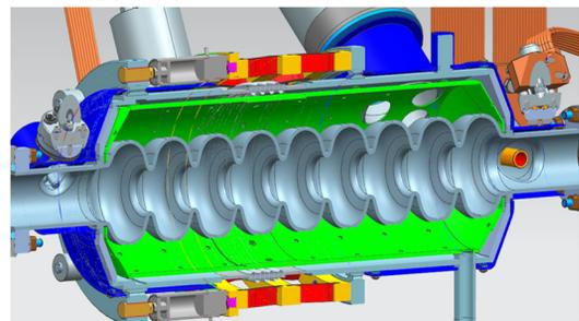
Figure 1: 3D CAD cross-section of a cavity with helium vessel.
