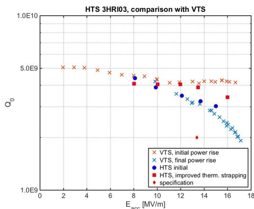
Figure 6: Comparison of  $Q$  vs  $E$  between VTS and HTS
