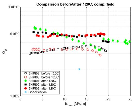
Figure 2: Q vs E performance in VTS, comparison of measurement before and after 120 C baking, cooldown in compensated magnetic field.
