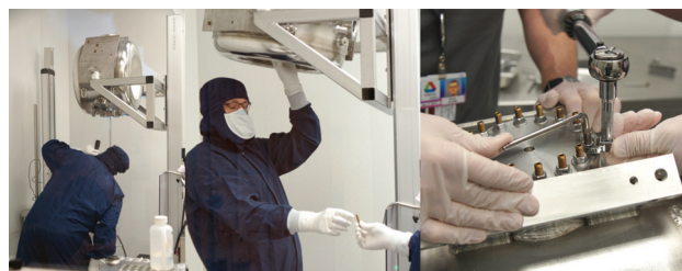
Figure 3: Vertical HPR, cavity assembling and tightening.
