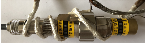
Figure 1: Coaxial line test fixture with Dezifix connector [10], PT100 sensor, heating braid and non-reversible temperature indicators.
