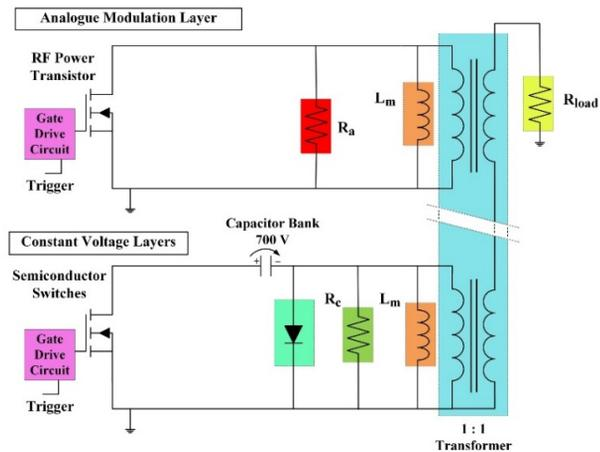
Figure 1: Schematic of an inductive adder with a single constant voltage layer with core loss resistance  $R_c$  and magnetizing inductance  $L_m$ , and with an analogue modulation layer with modulation resistance  $R_a$ , magnetizing inductance  $L_m$  and an RF power transistor.
