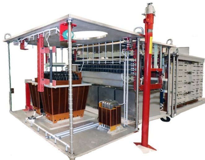
Figure 4: 250 MW Modulator construction, with the pulse transformer in front, and the switch modules at the rear. The energy storage capacitors are visible in the center section. This entire assembly is submerged in an oil tank for operation.
