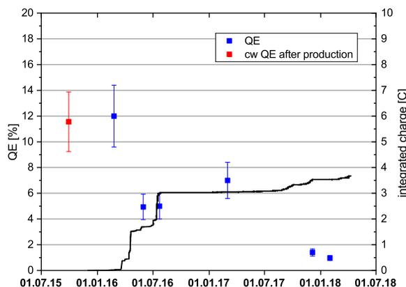
Figure 3: Quantum efficiency (blue squares) and integrated charge vs. time for cathode #680.1, operated at European XFEL. The red data point shows the QE right after production measured with Hg-lamp.
