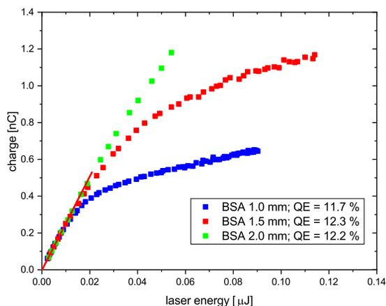
Figure 2: Charge as function of laser energy for cathode #680.1 for three different laser spot sizes (BSA) at the cathode, blue squares: 1.0 mm, red squares: 1.5 mm, green squares: 2.0 mm, red line: fit to the data as described in the text.
