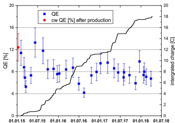
Figure 4: Quantum efficiency (blue squares) and integrated charge vs. time for cathode #73.3, operated at FLASH. The red data point shows the QE measured right after production with a Hg-lamp.
