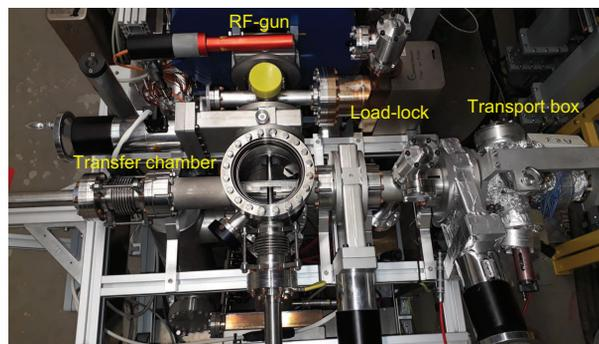
Figure 1: Cathode transfer system of the European XFEL. It is a copy of the FLASH system with a few improvements.
