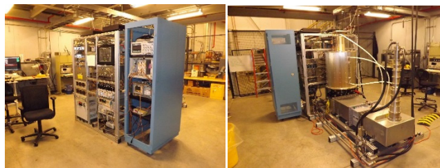
Figure 1: Left, front view showing operator controls and adjacent low-level rf control rack (blue). Right, rear view showing the cylindrical output combining cavity, waveguide transmission system, and terminating rf load.
