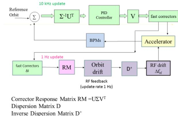
Figure 1: FOFB operation with RF correction (schematic).
