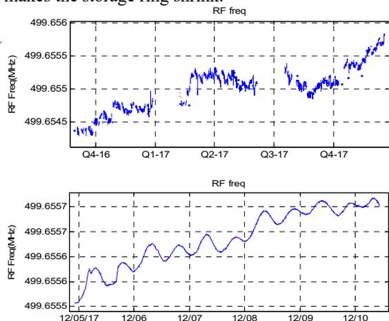
Figure 3: The upper plot is the RF frequency variation from September 2016 to December 2017 and the lower plot shows a more detailed observation for four days. RF variation per day is around 100 Hz, equal to path length about 100 µm.
