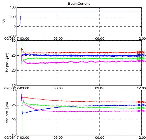
Figure 6: For the first 30 minutes of beam stored, orbit change could be up to 10  $\mu\text{m}$ . Then the horizontal could be stabilized while the vertical orbit still have slow drift (2~3  $\mu\text{m}$ ) for the first 4~5 hours.
