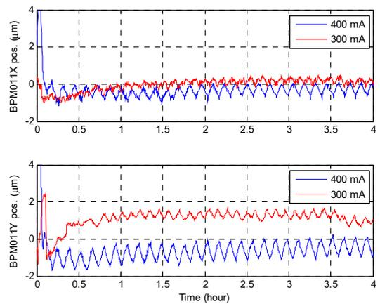
Figure 8: BPM position variation with beam current become to worsen when 400 mA top-up mode than 300 mA.
