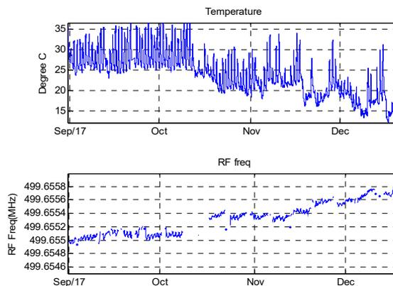
Figure 4: Seasonal temperature variation versus RF frequency changes. From October, the outside temperature of TPS site is decreasing while RF frequency is increasing. 10°C drop of the temperature would cause 400 Hz increase of RF frequency.
