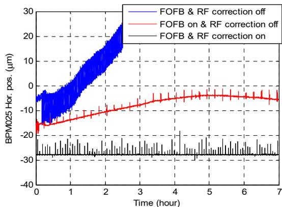
Figure 2: Orbit stability comparison with/without FOFB and RF path length compensation. The spikes are due to regular injection when FOFB and RF frequency correction is temporarily inactive.
