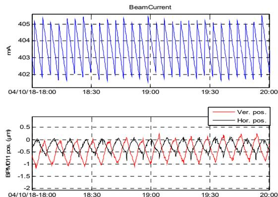
Figure 7: BPM position seems to have a small variation (less than 1  $\mu\text{m}$ ) with beam current at top-up mode, especially at the location of the injection section.
