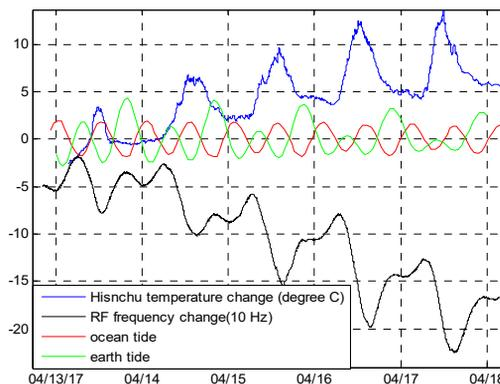
Figure 5: The black line is the RF frequency change while applying RF frequency corrections. The blue line is the ambient temperature on the NSRRC site. The red line is the ocean tide at the seashore about 15 km west of the TPS site provided by Central Weather Bureau of Taiwan [4] and the earth tides in green are calculated from the Program *solid* [5].
