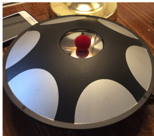
Figure 2: Mirascope with red ball inside at bottom and its image formed above the opening
