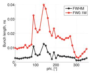
Figure 7: Predicted FWHM and FW0.1M bunch length using the Astra software [7]. In the simulations the shortest bunches are found around  $\phi_B \simeq 300^\circ$  and at that position the FW0.1M is much more sensitive to booster phase change than the FWHM.
