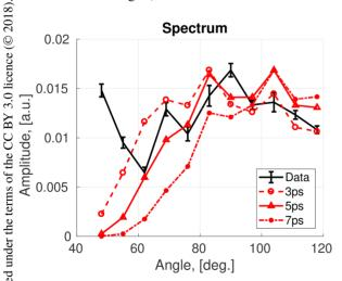
Figure 4: Example of measured spectrum as function of the 🛎 detector angle. The measured data are in black and the three gred lines give simulated spectrum for a bunch length of 3 ps FWHM (dashed line), 5 ps (plain line) and 7 ps (dot-dashed line).
