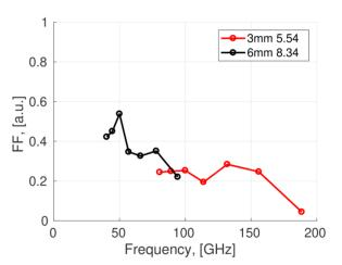
Figure 9: Form factors measured for two different gratings with different pitches.
