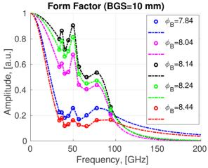
Figure 5: Form factors reconstructed for different settings of the booster phase  $\phi_B$ . The two data points above 100 GHz have been excluded as non-sensical. The recorded signal is represented by the open circles and the dashed line correspond to the interpolations between these points and the extrapolations outside the sensitivity range as described in [6].
