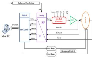
Figure 2: The LLRF control system for Buncher.
