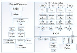
Figure 3: LLRF block diagram of buncher.
