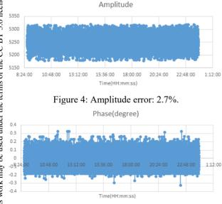
Figure 5: Phase error:  $\pm 0.32^{\circ}$ .
