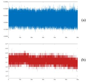
Figure 9: The amplitude (a) and phase error (b) of SC LLRF.
