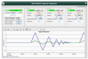
Figure 8: Interface for Python-based degaussing program.
