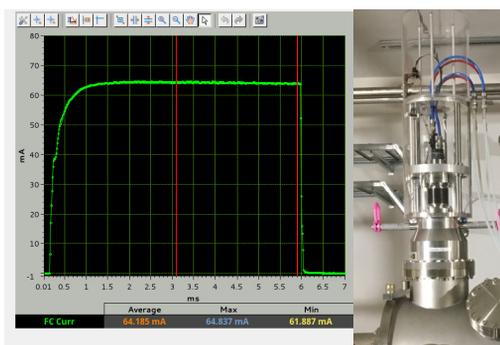
Figure 10: FC commissioned in Catania and in LEBT at ESS tunnel.
