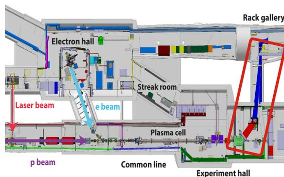
Figure 1: Layout of the AWAKE experiment. The part highlighted in red shows the spectrometer system.
