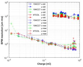
Figure 4: Resolution of button BPMs with E-XFEL Feed Throughs (old/new).
