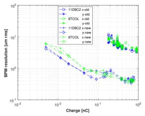
Figure 3: Strip-line BPM resolution (old/new).
