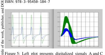
Figure 5: Left plot presents digitalized signals A and C ŝ directly from pickup. Extracted bunch informations from 1 author ms data acquisition (ADC data) is presented on the right plot (~1900 extracted bunch signals are ploted).
