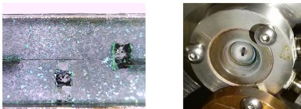
Figure 2: (left) original in-air pinhole assembly (Tungsten slits) saw corrosion, after a short period of 50mA operation. (right) white/green powders deposited at the diamond window.
