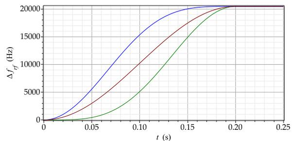
Figure 4: Rf frequency program for the Booster, injection on-momentum and extraction at  $\delta p/p = -0.006$ . The maroon curve has no path-length correction, the green curve has the most negative correction and the blue curve the most positive correction.
