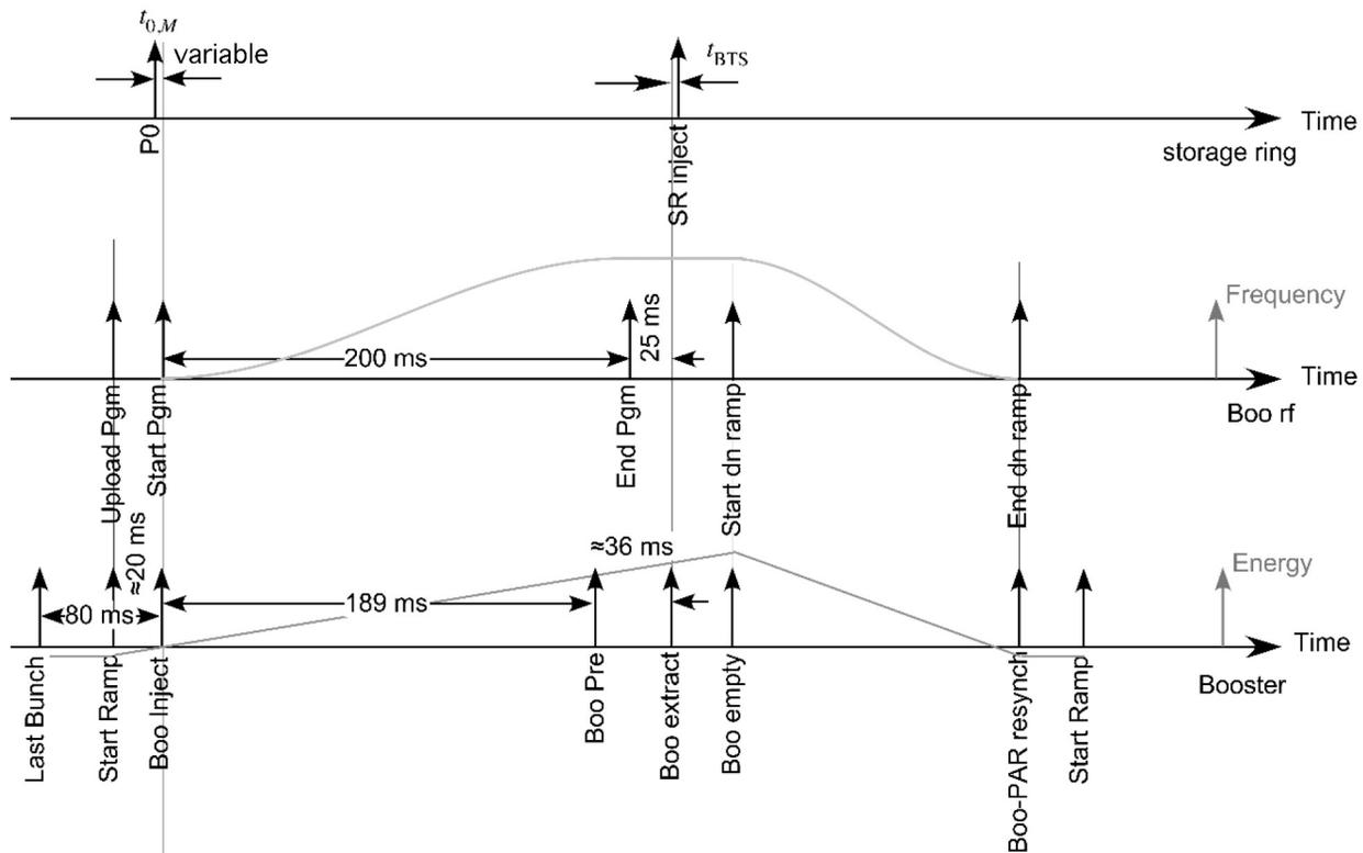
Figure 5: Timing fiducials. Start Ramp initiates the Booster B-field ramp; Upload Pgm indicates calculation of the frequency ramp and upload to the DDS controller; Start Pgm indicates the start of the frequency ramp play-out. Injection and extraction happen during the B-field ramp.
