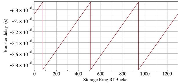
Figure 3: Booster path-length correction time  $\delta t$  vs the MBA bunch number injected into.
