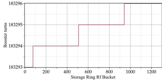
Figure 2: Number of Booster turns vs the storage-ring bucket to be injected into.
