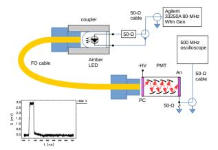
Figure 4: FO transmission test schematic. Inset shows the PMT output test pulse at a bias of -400 V.
