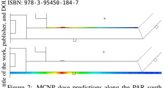
Figure 2: MCNP dose predictions along the PAR south author(s). shield wall for 2 nC, 500 MeV beam loss. Top: inside  $e^+/e^$ dose, peak: 6.1 mrem; bottom: outside photon dose; peak: 0.095 mrem. See Fig. 1 for geometry reference.
