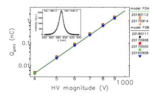
Figure 5: Prototype FO cable transmission with HV bias over the last two years of running. Inset shows the LED spectrum used for these measurements.
