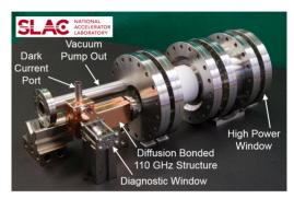
Figure 1: Components for the high power test assembly prior to final fabrication. The diffusion bonded copper accelerating structure is shown in the foreground. The high power pulse enters from the right through a window (not visible). The diagnostic port allows for calibrated transmission data which provides an accurate measurement of the fields in the structure.
